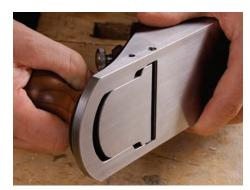
**Adjustable mouth.** Changing from a narrow opening for light shavings to a wide one for heavy work is quick and simple because you don't have to move the frog, as you would on traditional bench planes.
