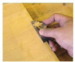
▲ ...or on its side for shoulder trimming on the push stroke
