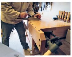
▲ ...or the jaws can be used conventionally to clamp workpieces solidily to the bench while you work them
