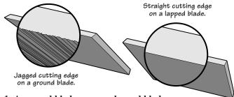
Figure 1: A ground blade versus a lapped blade.
