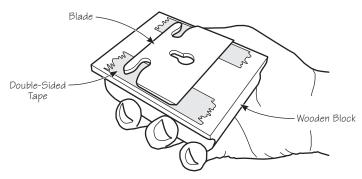
Figure 4: Simple blade holding jig.
