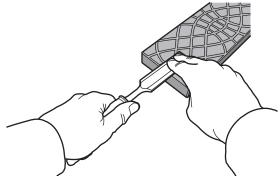
Figure 6: Lapping a chisel.
