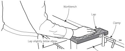
Figure 7: Lapping set-up.
