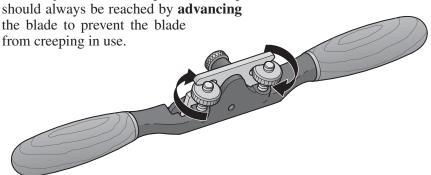
Figure 2: Turn thumb wheels to set the depth of cut.
