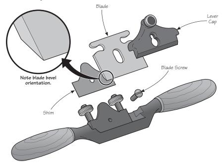
Figure 4: Using shims to adjust the mouth.
