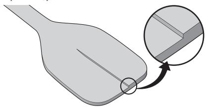
Figure 5: Blade corner may dig into the workpiece.
