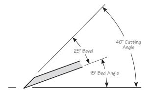
Figure 3: Blade geometry as supplied.
