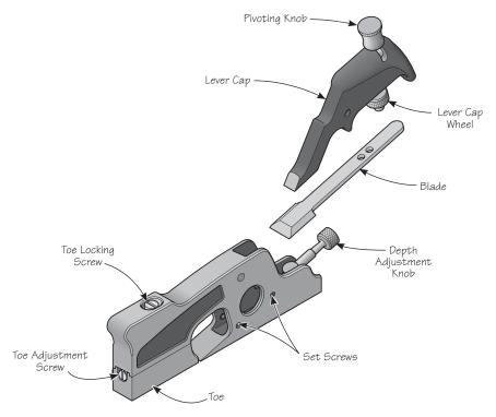
Figure 1: Shoulder plane components.
