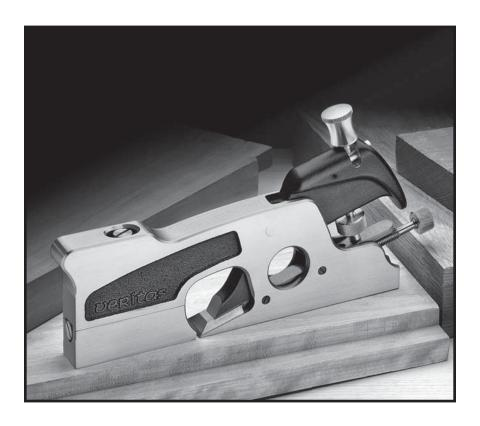
The Veritas® Medium Shoulder Plane is proportioned to handle multiple tasks, from fine trimming shoulders for a perfect fit to cleaning the bottom of dadoes. It measures 7" long by 0.700" wide and weighs just over 2 pounds. The ductile cast iron body is accurately machined and ground so that the sole and sides are flat and square, allowing the plane to be used on its side for accurately shooting the shoulder of a tenon.
