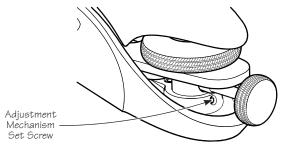
Figure 3: Set screw that holds the adjustment mechanism in the body.
