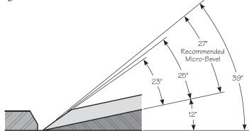
Figure 7: Recommended blade geometry of the low-angle block plane, with a  $27^\circ$  micro-bevel.
