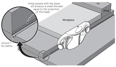
Figure 6: Planing end grain with the block plane.
