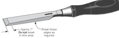
Figure 4. Breaking the side edges.
