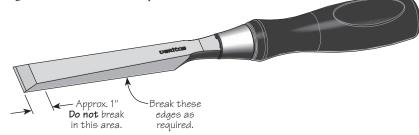
Figure 4. Breaking the side edges.
