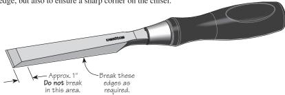
Figure 4. Breaking the side edges.
