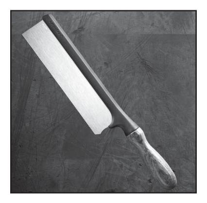
The Veritas<sup>®</sup> saws combine the best characteristics of the classic gent's saw with those of state-of-the-art materials and construction methods. The tooth pattern on the thin high-carbon steel blade provides a good balance between cutting action and surface finish. The stainless-steel/glass/polymer composite spine provides strength and rigidity.
