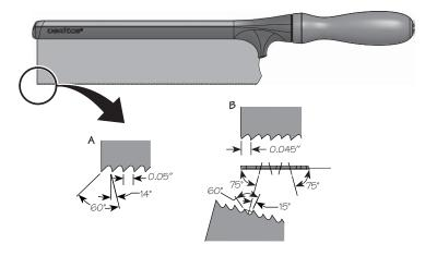
Figure 2: Sawtooth geometry for rip (A) and crosscut (B) gent's saws.
